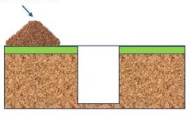
The soil is in its natural state, uncontaminated and will not leave site. The team have deemed material suitable for reuse for the specification they are working to, but additives are required to change the chemical and/or physical properties. This may be classed as waste treatment and a permit maybe required. Seek further advice. A SWUK Site Assessment is required before commencing with adding additives and only Green (Non-hazardous) material can be reused.
