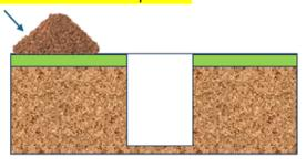
The soil or NOM is in its natural state, uncontaminated and will not leave site. The team have deemed material suitable for reuse for the specification they are working to, but additives are required to reduce moisture content.
