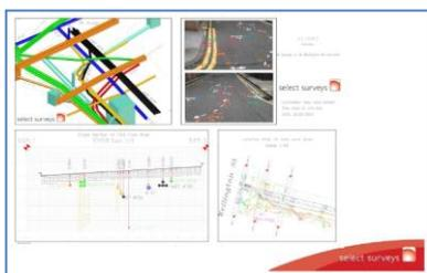
Augmented Reality technology using underground asset data supplied by clients, smartphone cameras and GPS functionality to display data such as maps, tags and images, are used to determine realistic uses for AR (e.g. pre-site surveys). Using a phone's built-in GPS, the software calculates the phone's location and overlays the asset data. Images show water (blue) and gas (red) mains and kerb line (purple).
